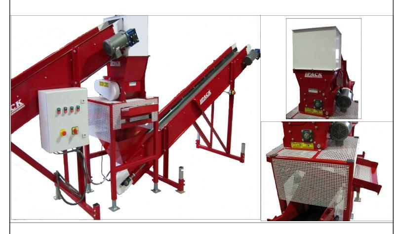
Pack Manufacturing Media Recycling Processor is designed to help growers conserve growing media by recycling used materials. This machine uses a mill type processor to break up roots and dislodge potting soil. A cleated incline conveyor delivers the media to the processor. After the material is processed it continues onto a vibrating screen that separates the unwanted portion and allows the balance to drop onto another conveyor for reuse.
