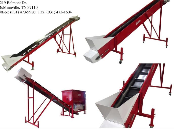
All Pack Manufacturing Conveyors are built with self-tracking belts and sealed bearings to minimize downtime and machine maintenance. Direct drive gearboxes are used instead of chains and sprockets to provide a safer, more solid design. Pack Manufacturing Conveyor Lines can be finished with custom hoppers and end dump chutes to fit your needs.
