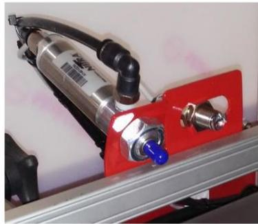
Photo Eye Sensor w/ Delay Arm
