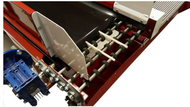
Direct Drive Conveyor with Soil Return Chute
