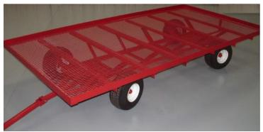
Pack Manufacturing Tracking Wagons are our highly affordable solution to field mobility. Whether transporting labor, products, or equipment, a Pack Manufacturing Tracking Wagon will be up to the task. Our Tracking Wagon series varies greatly depending on need and application, but all Pack Manufacturing wagon lines are built with a heavy-duty angle iron frame and a flattened expanded metal bed. Our Tracking Wagons are built to hold up under extreme conditions and made to last a lifetime.
