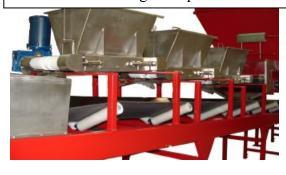
Self-Tracking, Low Friction V-Roller Belts deliver media components quickly and efficiently. Integrates easily with soil processing attachments and automated potting lines.
