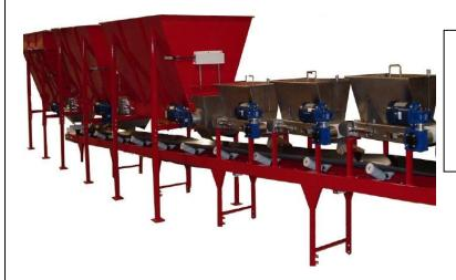
Alternate Bulk Hoppers store the large volume components, like peat moss or sand. Pack Manufacturing Bulk Hoppers are constructed of heavy-duty steel. Options include low-level sensors, covers and custom chutes. Low-level sensors can alert or automate hopper refills.
